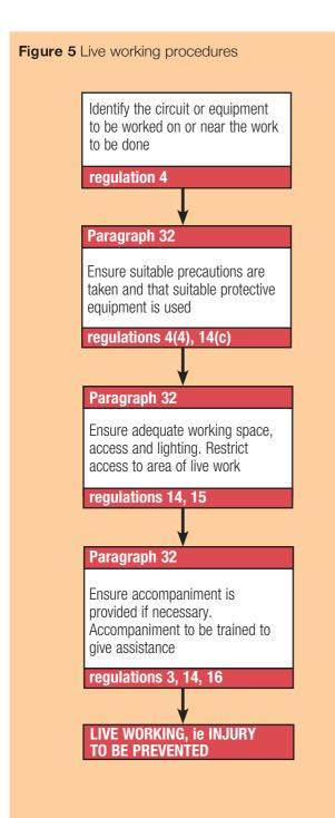
85 The procedures associated with live working are illustrated in Figure 5. While it is not always possible to follow rigidly a set procedure to cover all situations, you should follow the management principles described in this guidance and the safe system of work criteria set out in paragraphs 25–32.
